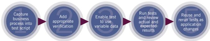
WinRunner emulates and captures user actions into test scripts that can be used throughout the application's lifecycle, using the above process.
